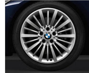
■ 18" light alloy wheels Multi-spoke style 416 , 8J x 18 with 225/45 R18 tyres.
