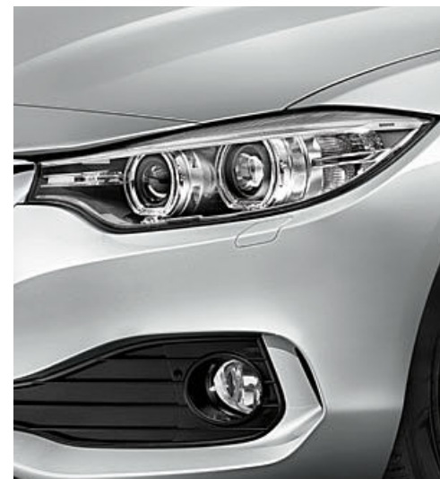
Xenon headlights with low-beam and high-beam function come as standard and also include headlight washer system, LED accent light, automatic headlight beam range control and four LED light rings that act as parking lights, side lights and daytime driving lights. Foglights in the front apron are included as standard and increase safety in bad visibility.
