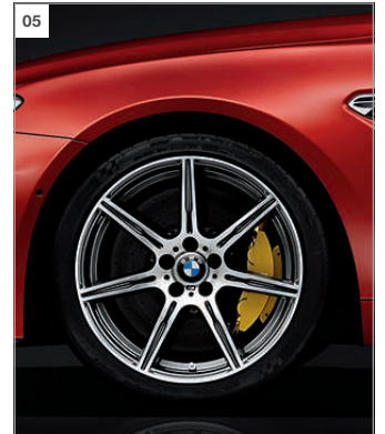
[ 05 ] 20" M light alloy wheels Double-spoke style 601 M (optional), Bicolour, gloss-lathed, with mixed tyres. Front: 9.5 J x 20 with 265/35 R 20 tyres. Rear: 10.5 J x 20 with 295/30 R 20 tyres. 2
